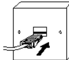
Use the plug to raise the shutter before pushing it into the socket
